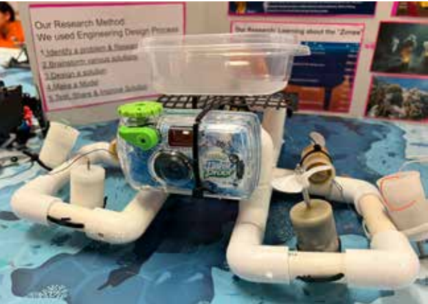
Underwater Robot model equipped with a camera was designed by students to study deep water ecosystems. Emma Hughes/GRIN
